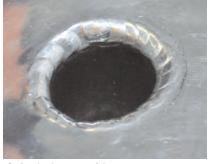
Curiously, the power of the vacuum pump can deflect the top skin of the alloy valve covers enough to propagate a crack around the plug holes. Welding the crack is not without its troubles. Invariably another crack will develop beside the weld.
