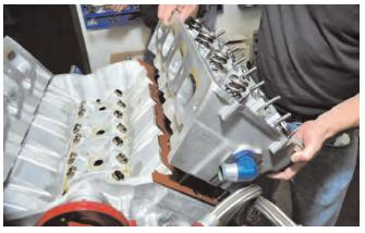
Copper spray from an aerosol can is applied to the top and bottom surfaces of the three-layer Cometic head gaskets, then the heads are fit and tensioned to 130-140 ft-lb.
