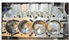
The diameter of the forged pistons usually measures 4.770 inches. The small-bore holes around the perimeter of the CP pistons are gas ports. These allow combustion gases to enter the top ring grooves, imposing a force on the inner edge of the top rings and forcing them out onto the cylinder walls.
