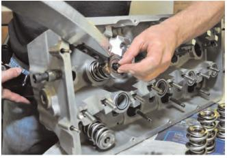
Next, the triple valve springs are laid out for installation. Hardened seats are fit between the spring and the aluminum head. Oil is applied to the valve stems and the valves are inserted into the cylinder head. Aided by a pneumatic valve spring compressor, the locks are carefully sandwiched between the valve stems and the retainers.
