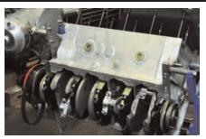
The mighty Bryant billet crankshaft resides in the aluminum block and functions with aluminum rods, bearing caps and main caps. Aluminum is lighter than steel, and it makes accurate line boring easier. When honing dissimilar metals, the hone is inclined to push toward the softer metal.
