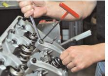
Pushrods are installed, SS billet rockers positioned, their shafts tightened to 35 ft-lb and valve lash adjusted for engine warming on the dyno. Usually the clearance between the exhaust valve and the rocker is zero, and the clearance between the inlet valve and the rocker is 1/8th of a turn from tight. In this way, when the engine warms the inlet, valve lash will measure 0.030-inch and the exhaust 0.020-inch.
