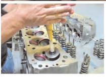
The first part of the process of installing the valves is to check the continuity of the seal between the valve head and the valve seat. This is accomplished by applying red dye to the seats and lapping the valves into them. If continuity is broken and traces of red dye remain, the offending seats will be recut. Both inlet and exhaust valves are made of titanium. The diameter of the inlet valve measures 2.680 inches and the exhaust measures 2.040 inches.
