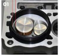
01. The head of the 2.100-inch intake valve maintains stems measuring 11/32x5.450 inches, the stems of the 1.600-inch exhausts are 11/32x5.460 inches.
