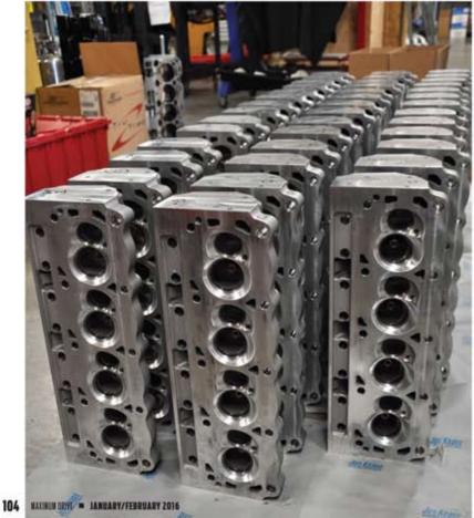
08. The P38 cylinder heads have a mounting provision (2-inch centers) for conventional tubular exhaust headers as well as wider (3 inch) centers that allow for larger exhaust ports.
