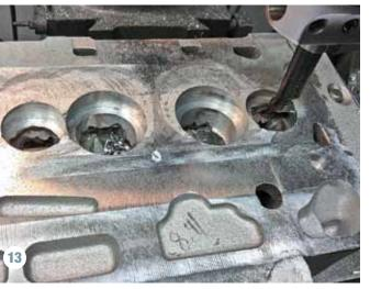
Kaase knew approximately where the valves would be located, so he installed a head in a Bridgeport machine and cut the seat registers and drilled tentative valve guide holes. The angle of the spark plug wouldn't change significantly, but its final location would be positioned much deeper in the head.
