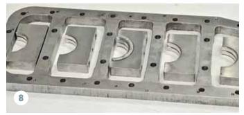
Cleverly, the main cap girdle was produced from one-inch-thick 1045 steel, and the main bearing caps were created by claiming and machining the sections of steel cut out to form each of its five windows—a process known as nesting. A series of long, 1/2-inch head studs from another engine, probably a Ford Cleveland V-8, and 20 perimeter bolts were used to unify the crankcase, mains caps and girdle. The medium tensile carbon steel known as 1045 is typically used in the construction of mains caps.
