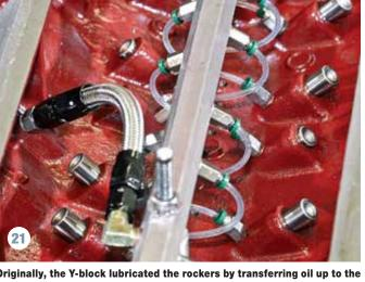
Originally, the Y-block lubricated the rockers by transferring oil up to the cylinder head and through the one-piece rocker shaft. But the system used on this EMC engine was altered; Oil was diverted to the tappets. which were equipped with an internal oiling system that moved the lubricating oil northward to the rockers via the tubular core of each pushrod.
