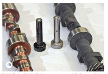
For the Engine Masters Challenge, a steel camshaft (left) was employed. After the contest, a cast-iron camshaft was substituted to test the engine for peak power. Both camshafts used tool steel tappets with DLC ("diamond-like carbon") coating being applied to those operating with
