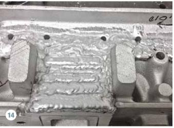
Notice how the depth of the cylinder head has been increased by approximately 1/4 inch at the rocker cover mating surface. Also, observe the sea of aluminum weld metal, which will provide sufficient material to raise the entry of the intake ports and introduce adequate substance to accommodate machining of the port roofs.
