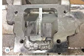
A dividing wall of a new Siamese port is cut, inserted and welded in place.
