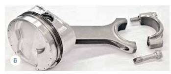
Still, Kaase was limited to 0.345-inch lobe lift. To do otherwise would have meant grinding more material from the connecting rods and thereby weakening them further. Consequently, he decided to make up the valve lift deficit by increasing the rocker ratio to 2.0:1.
