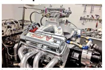
In a more street-friendly configuration running a shorter intake and single four-barrel, Kaase still managed to reach 700 hp.
