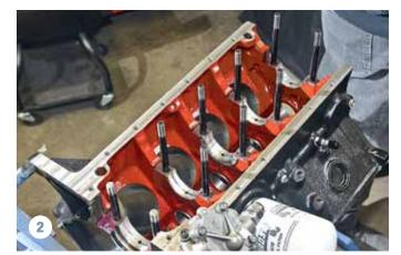
The term "Y-block" means the lower regions of the block structure don't end at the crankshaft centerline, but instead extend further downward. their deep skirts introducing strong bulkheads or webs that support the main bearings. In the second half of the twentieth century, Y-block configurations were popular with several car companies; today the Chevrolet LS-series V-8 engine is a prominent example.
