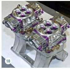
The carburetor company CFM is owned by Dale Cubic, whose main carburetor bodies are constructed of billet aluminum. Cubic supplied Kaase's carburetors, whose chief draw sufficient fuel at low engine speeds. "I didn't want it to go lean at 3,000 RPM."
