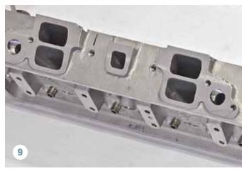
Two sets of cylinder heads were acquired. One set of original heads was purchased in an online auction. These were sacrificed in a quest to ascertain the layout of the water jackets. "I'd never known an engine with upper and lower intake ports," says Kaase.
