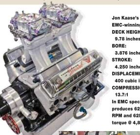
**EMC-winning Y-block DECK HEIGHT:** 9.78 inches BORE: 3.876 inches STROKE: **4.250** inches DISPLACEMENT: 400 cubic inches **COMPRESSION RATIO:** 13.7:1 In EMC specification it produces 620 hp @ 5,800 RPM and 625lb-ft of torque @ 4,800 RPM
