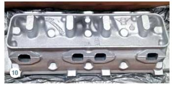
The other set of heads was purchased from Y-block specialist John Mummert (www.ford-Y-block.com), These were raw unmachined castings. Because Y-block heads feature more turns and, therefore. are more difficult to port, Kaase decided to convert the Mummert head castings to conventional intake ports. "A shining flashlight at the port entry barely penetrates the other end of the Y-block heads," he notes.
