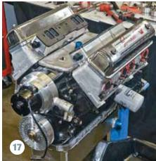
To gain optimum nduction flow. a high-rise manifold was acquired. The Edelbrock 7110 Street Tunnel Ram for a small-block Chevrolet (SBC) was selected. But because the deck height (that is the dimension from the crankshaft center line to the upper deck surfaces) of the Chevrolet differed by approximately 0.780-
