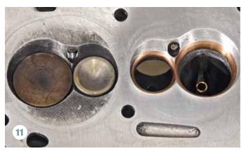
Kaase not only modified the combustion chamber as suggested by the faint weld line still visible on the finished result shown here, but also changed the depth of the chamber and moved the valve locations. Valves were made from blanks obtained from Ferrera. "The stems are already finished, and I introduced valve lock grooves and machined the valve heads to the finished sizes: 2.08 and 1.54 inches."
