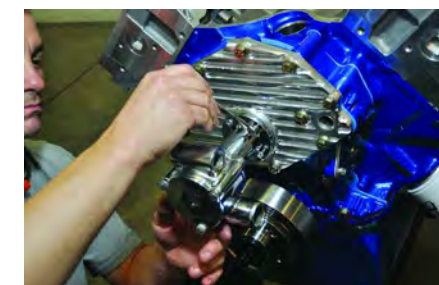
17. Installing cam - Installing cam-driven Magnaflow water pump.
