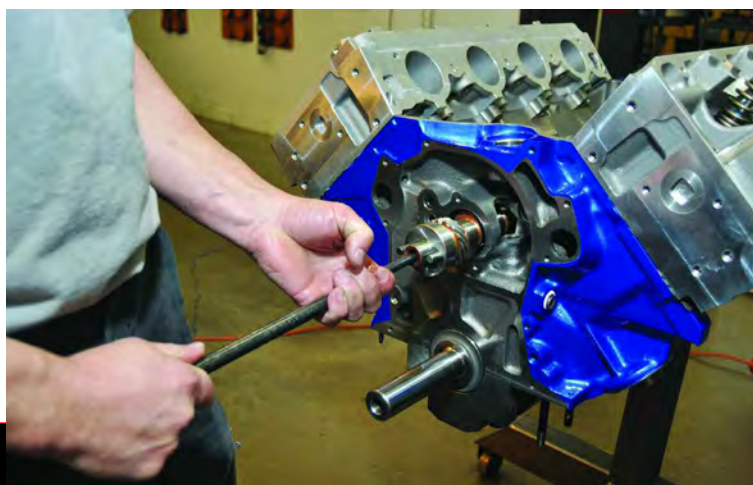
11. Inserting camshaft - Temporary "handle" aids easing the lubed-up camshaft through the galley taking care not to nick the cam bearings with the lobes of the camshaft.
