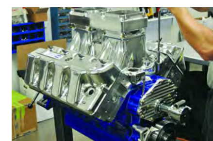
19. Adding the manifold - There are several intake adaptations for the Boss Nine, a single 4150 or 4500 Holley on a single-plane intake manifold, tunnel ram with twin 4150 or 4500 carburetors, Hilborn stack fuel injection, a BDS supercharger set-up, or a Wilson four-barrel EFI system that offers 1388cfm. The Boss Nine is also available with a 1-inch Wilson spacer beneath a Dominator-style carb that improves airflow by 130cfm.
