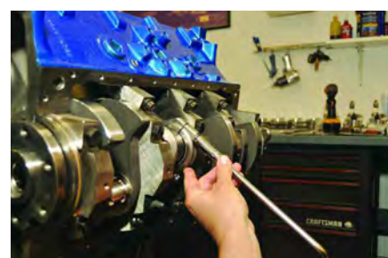
9. Securing rods - Caps for forged steel Scat connecting rods are secured with 12-point Grade-10 bolts and torqued to 75lb/ft.
