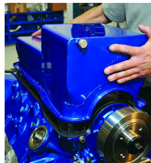
16. Installing oil pan - Boss Nine engines are equally adaptable to either dry- or wet-sump oiling. This wet sump application uses a Moroso 7-quart pan featuring three main components: a one-way mesh screen bolted to the sump, a 3/4 inch wide metal scraper that runs the length of the pan and is mounted at the top of the mesh screen, and two one-way trap doors in the pan itself. The traps act as a check valve, in that they allow oil to enter the lower regions of the pan but not readily escape. A Kaase oil pump (blueprinted, welded pick-up, etc.) replaces the stock unit that inevitably fails under duress.
