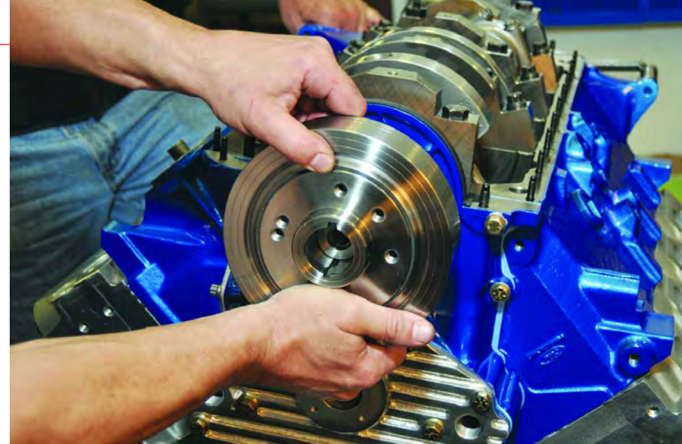
14. Installing harmonic balancer - Internal engine parts when in motion become out of balance and induce vibration. The harmonic balancer is an SFI approved weight (not a pulley) that attaches to the front end of the crankshaft and absorbs vibrations. For a tight fit on the crankshaft Kaase installs it with the power of a hydraulic ram.
