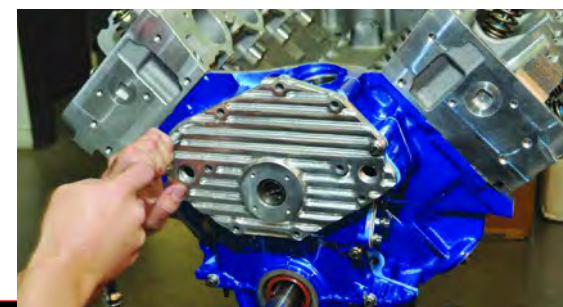
13. Installing WP cover - Kaase builds redundancy in this Boss Nine. The front cover encloses timing gear and chain and an optional eccentric fuel pump drive (as requested by owner). The ribbed alloy cover provides mountings for a cam-driven Magnaflow water pump.
