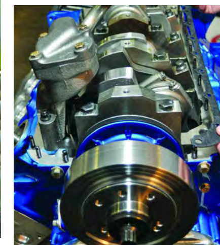
15. Adding oil pan gaskets - Oil pan rail gaskets are installed in anticipation of the sump.
