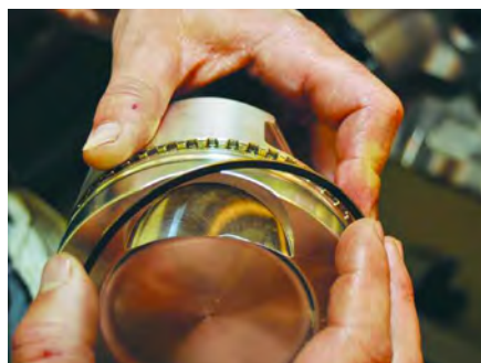
7. Assembling piston - Diamond 2618 forged pistons are outfitted thusly: the lower support rail of the oil control ring (bottom) is installed and followed by the upper support rail, the second ring, and the compression ring (top). The piston pins are made by Trend and hewn from the toughest tool steel H-13.
