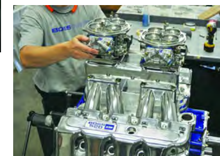
20. Carburetors - At the owner's request, this 528ci engine does swell with a tunnel-ram intake manifold and twin 4500 carburetors.
