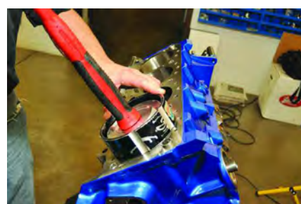
8. Installing pistons & rods - As always, a ring compressor and the butt of a mallet are used to carefully tap the oiled piston/rod assembly into the bore. Rubber guards on the rod fasteners keep threads from accidentally damaging crank journals.
