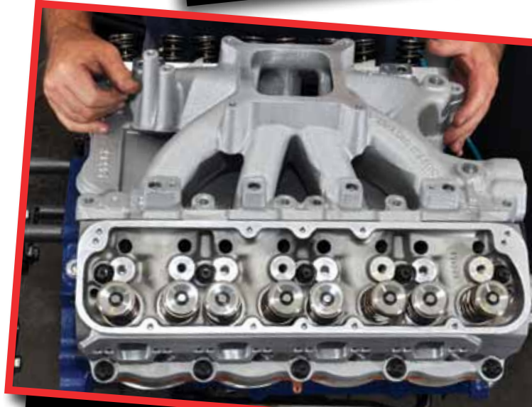
The P-38 conversion accepts any Windsor intake manifold, including EFI types, but the Edelbrock Super Victor and Victor Jr. have proven the most effective so far
